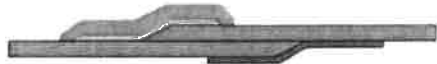
▶ Overlap seam with clear cover strap, PVC cover strap and seam tape
